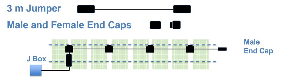
If the short cable (female) is to terminate into the J-box, you will need a male jumper and male end cap to complete the branch.
