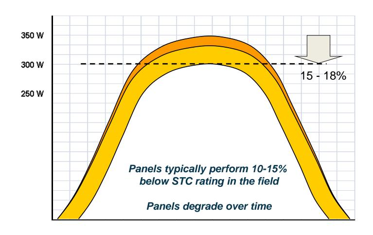
PV modules are typically oversized by 15-18% of inverter capacity with respect to their STC rating.
