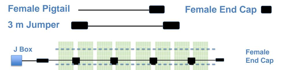
Use a pigtail to connect the long cable (male) into the J-box. Terminate the branch end with a female end cap.
