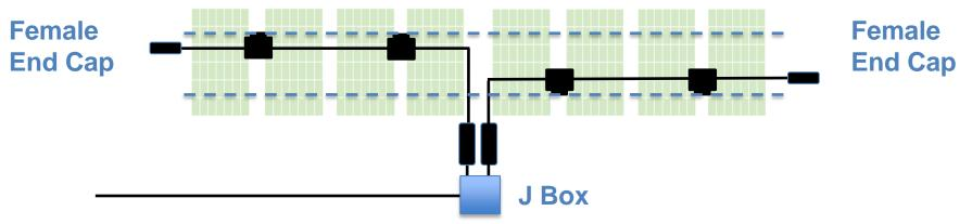
To center tap, use two pigtails to connect the long cables (male) into the J-box. Terminate each branch end with a female end cap.
