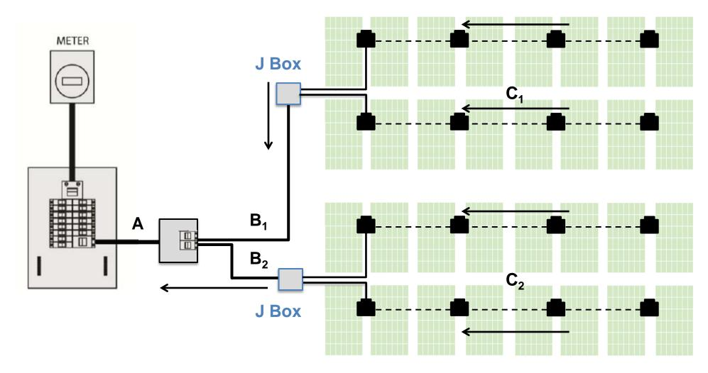
Two fully populated branch circuits equals 16A @ 240V for "B" and 32 A for "A" Center tapping allows "B" up to ~100' (10AWG) and "C" up to 10" (8 AWG)
