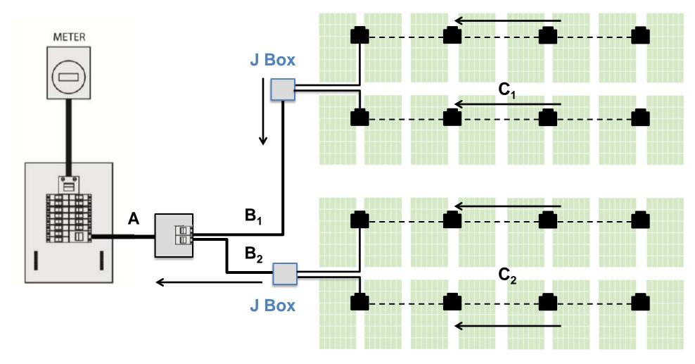
By center tapping, "C" now drops to 0.5%. Appropriate AWG wire sizing for "A" and "B" can be determined via a voltage rise/drop calculator such as:
